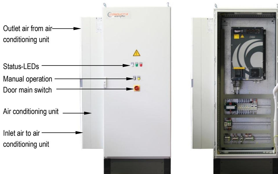
Fig. 3: Variant with air conditioning - view with closed and with open door
