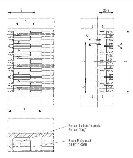
8-pole "End Cap Set complete" without power feed is shown. (8-pole "End Cap Set complete" = End cap set + 8 pcs. end caps for transfer points/end cap "long").
