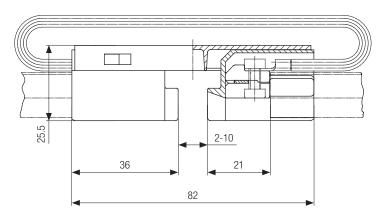
Expansion joints delivered with connection cables in different lengths.
