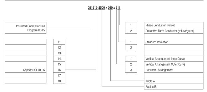
**Example:** Insulated Conductor Rail Program 0815;  $R_2 = 2500 \text{ mm}$ ;  $\alpha = 90^\circ$ ; vertical Arrangement (Outer curve), standard insulation, phase, copper rail 100 A. Part No.: 081516-2500x090x211
