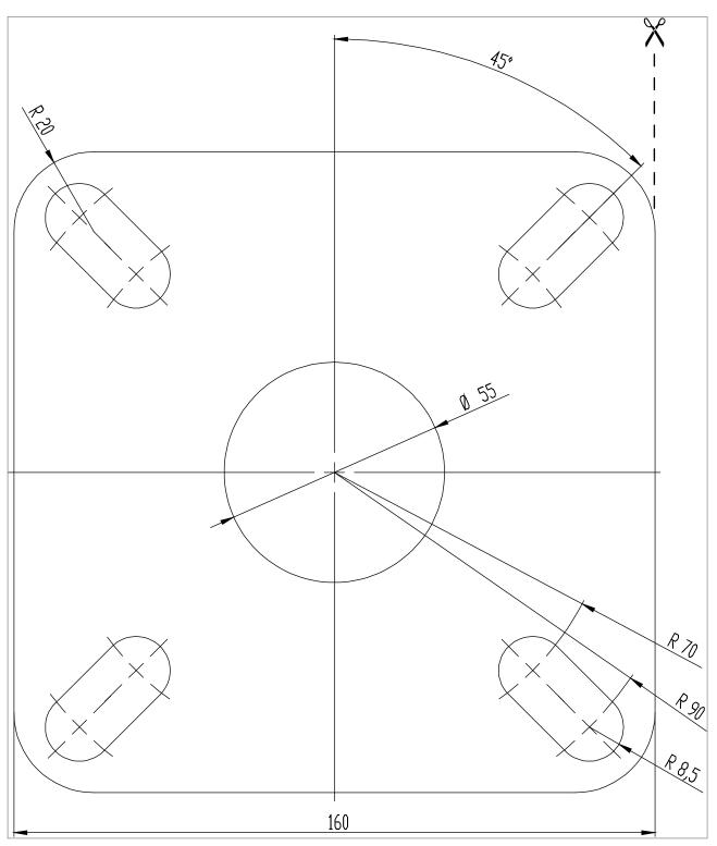
Fig. 6: Drilling Template BEF400 – 500/61-F001-0056
