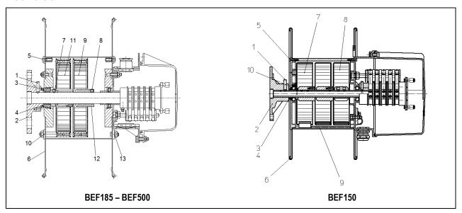
Fig. 26: Changing Springs, Series Connection with left Take-off
