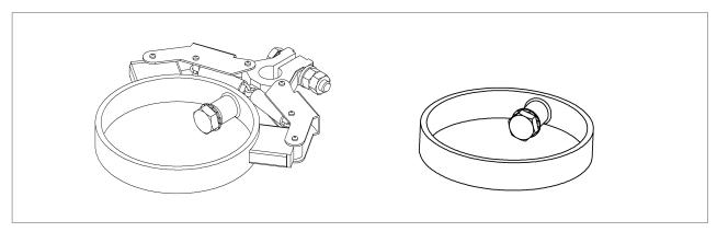
Fig. 20: Type 15, Current Collector with Slip Ring
