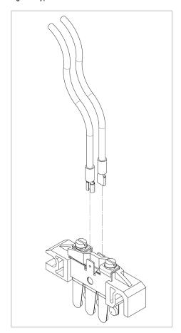
Fig. 13: Types 18 Current Collector Connection with Blade receptacle
