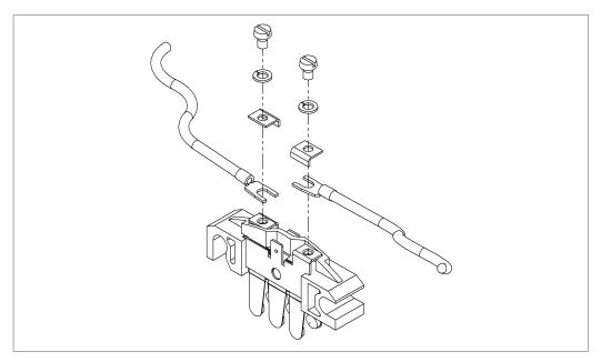
Fig. 12: Type 18 Current Collector Connection
