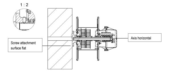
Fig. 7: Fastening Flange and Reel Axis
