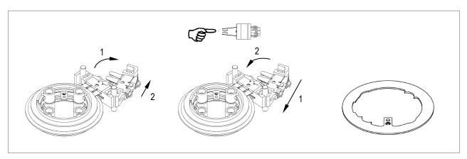
Fig. 22: Type 18 Current Collector, Assembly/Disassembly and Slip Ring
