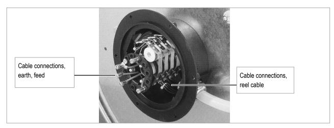
Fig. 8: Cable Connections on the Slip Ring Body
