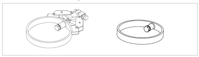
Fig. 19: Type 13, Current Collector with Slip Ring
