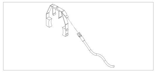
Fig. 9: Type 45 Current Collector Connection
