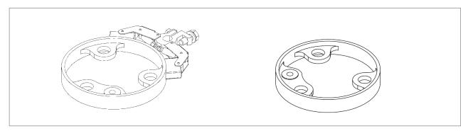
Fig. 23: Type 19, Current Collector with Slip Ring
