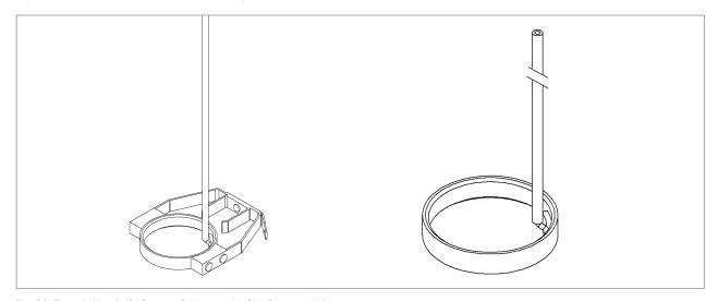
Fig. 24: Type 45/1 + 45/3: Current Collector with Slip Ring and Wire
