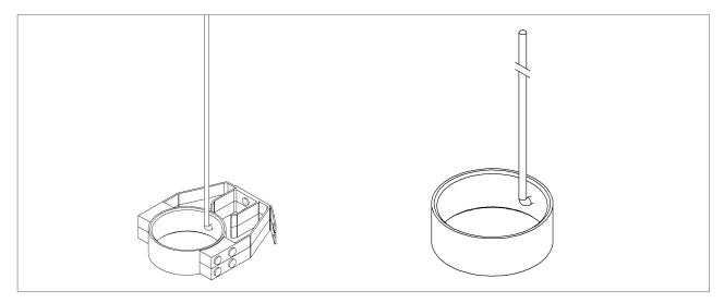
Fig. 25: Type 45/2, Current Collector with Slip Ring and Wire
