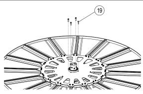
Fig. 7: Removing the 4 Cylindrical Screws
