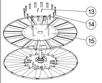
Fig. 4: Disassembly of the Spoke Wheel
