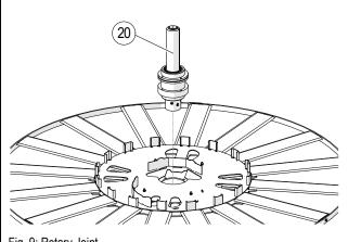
Fig. 9: Rotary Joint
