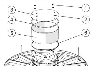
Fig. 2: Demount the Spring Housing
