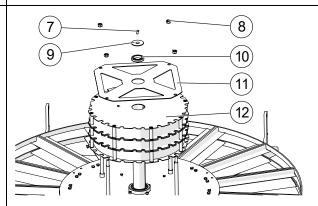
Fig. 3: Remove the Spring Cassette
