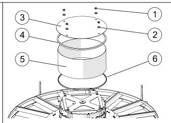
Fig. 5: Mounting the Spring Cassette
